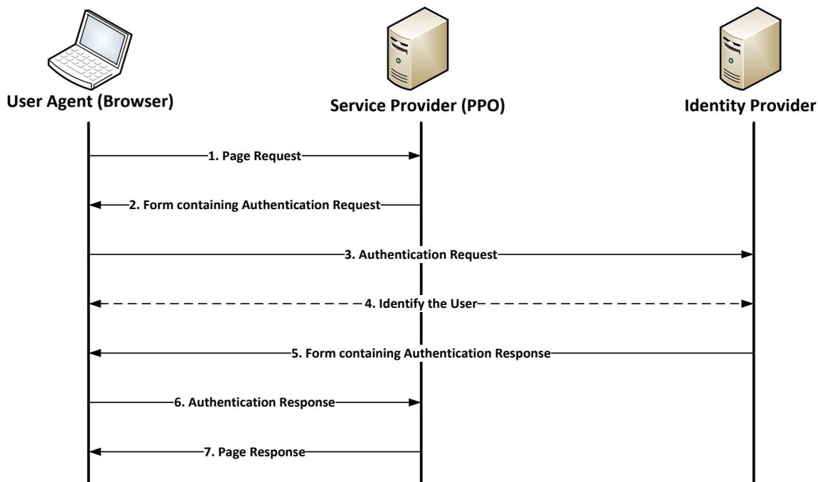
**Figure 1 – Service provider initiated SSO**
